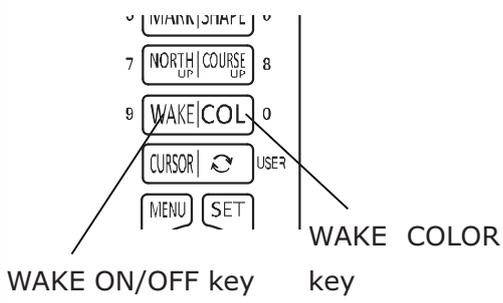
**1** Press WAKE ON/OFF key to start recording the wake.
