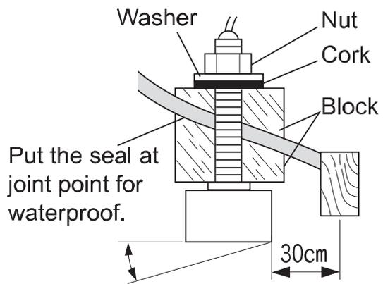
Keep the inclination of transducer surface below  $10^\circ$  or less.
