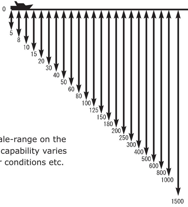
※This is only selected scale-range on the screen. The measuring capability varies depending on the water conditions etc.
