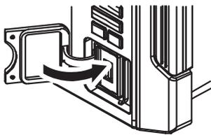
Put the slot cover firmly for water protection.
