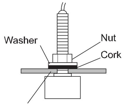
Put the seal at joint point for waterproof.
