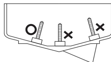
Do not install the transducer at the locations having obstruction like keel etc.
