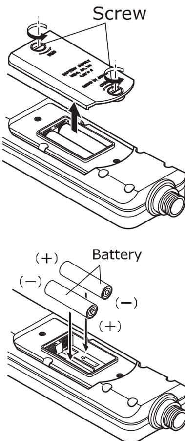
**1** Loose 2pcs screws and remove the rear cover.
