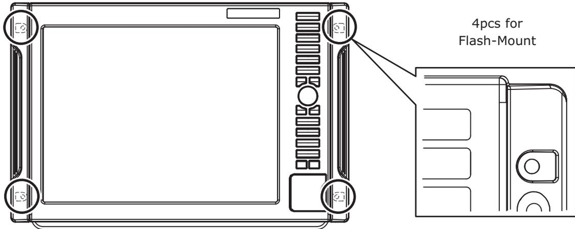
1. Refer to the following figure for fixation holes.
