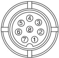
3. Connector for Water Temp Sensor
