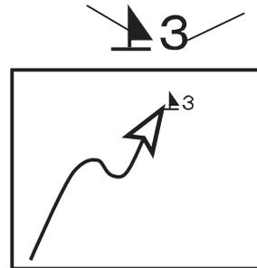
※When the cursor is ON, a waypoint mark is saved at the cursor location. When the cursor is OFF, a waypoint mark is saved at own vessel.
